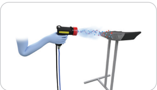
Headlight Cleaning With Airgun
