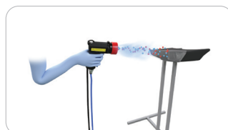
Headlight Cleaning With Airgun
