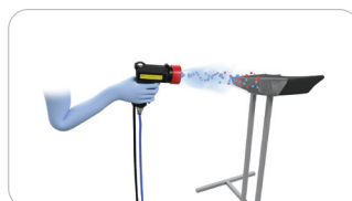
Headlight Cleaning With Airgun
