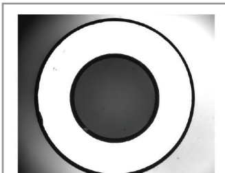
Edge defect detection, chamfer defect check on small metal parts
