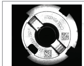
ID Read on metal part dot peen marked
