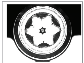
Concentricity measurement, part identification, part positioning
