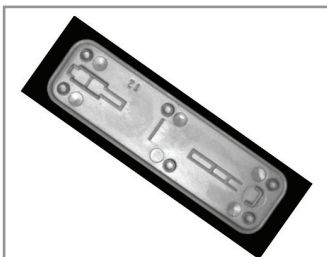
Missing part detection inside box, part positioning
