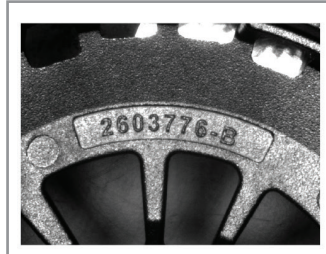
OCR on metal moulded parts, aluminium part defect detection
